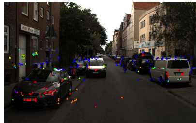
Colored by depth accuracy (red: accurate, blue: inaccurate).
