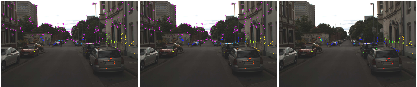
(a) Stochastic features colored by depth: red (close) to blue (distant); pink: no depth. (b) Interval features colored by middle depth: red (close) to blue (distant); pink: no depth. (c) Interval features colored by depth uncertainty: red (accurate) to blue (inaccurate).
