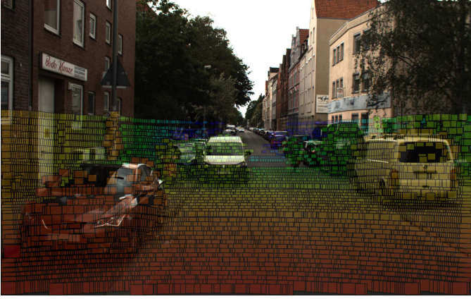
Fig. 4. Interval boxes enclosing the projected LiDAR points. The color of each box corresponds to the midpoint of the depth interval: from red (close) to blue (distant).
