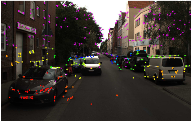
(a) Colored by depth: from red (close) to blue (distant); pink: no depth.
