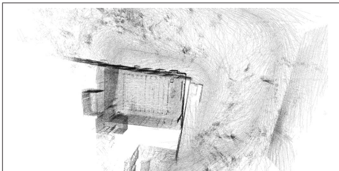
Figure 12. Map section generated by the SLAM approach for the lecture room dataset using an inappropriate timestamp offset between laser scanner and camera of 180 ms.
